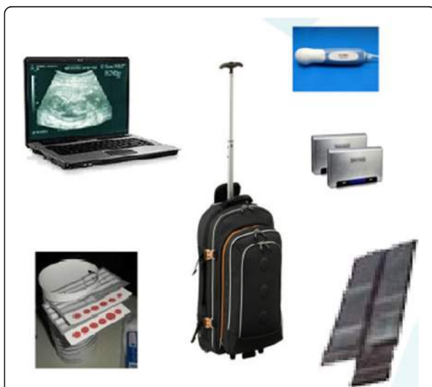
Fig. 1 Prenatal care kit elements: laptop, USB ultrasound probe, dried blood screening tests, backpack, external batteries and folded solar panel
