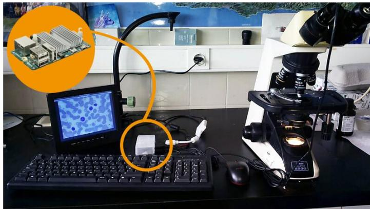
Figure 2. Telemicroscopy system with a detail of Odroid-U3
